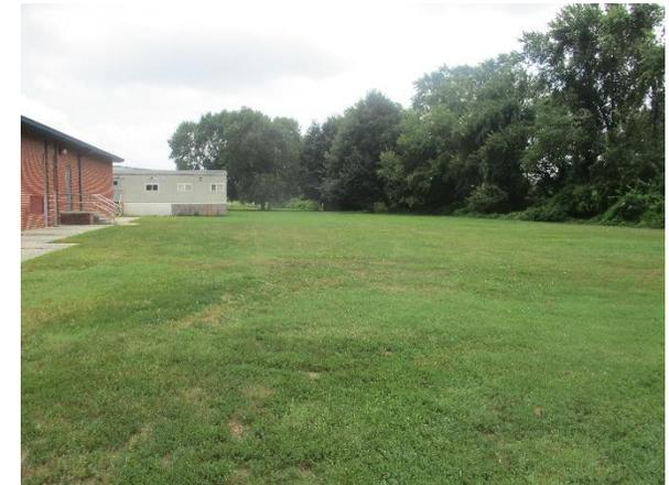
Bioretention systems may be installed to reduce stormwater runoff and can be used as landscaping for the school. A cistern near the mobile classroom can capture rainwater that can be reused for irrigation or classroom functions. A preliminary soil assessment suggests that more soil testing would be required before determining the soil's suitability for green infrastructure.
